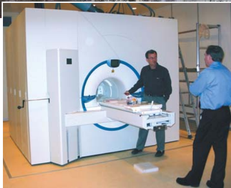
Magnex MRBR 7.0 T/680 mm, zero boil-off, active shield MRI magnet system.
