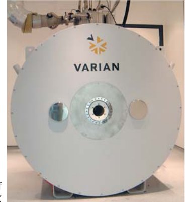
9.4T 210mm zero boil off magnet installed at Oxford, UK
