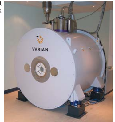
7.0T 310 zero boil off magnet installed at Edinburgh, UK
